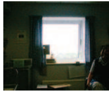
Figure 4.64 Window walls can appear to be very dark with light streaming in from a window. Capturing light by the use of reflective surfaces nearby can alleviate some of this contrast. The dark–light adaptation problems for visually impaired people can be extreme in this situation. Extra care with colour and lighting for window walls can help alleviate this contrast
