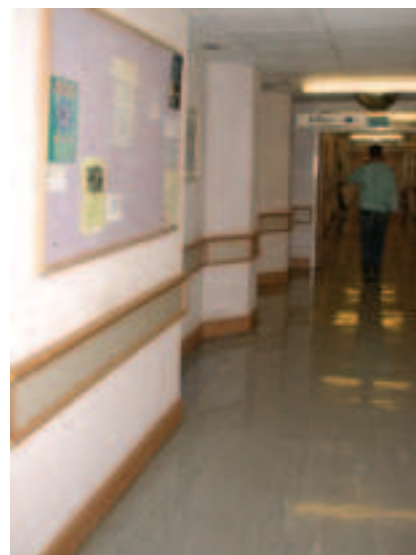
Figure 2.45 Colour used for navigation on or below dado rails could be particularly useful for all users of the environment
