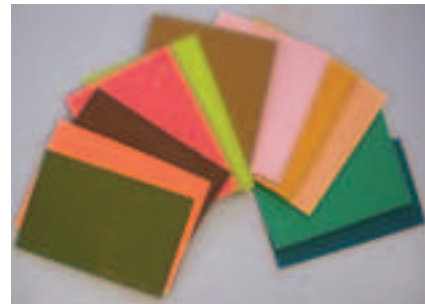
Figure 2.57 British Standard colours tend to reflect past interior colour trends however they are a useful standard for areas requiring regular repainting schedules
