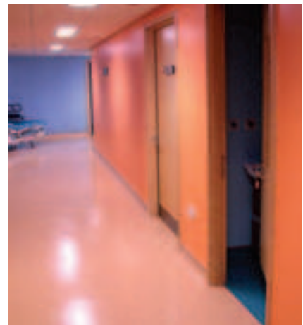
Figure 2.11 A more imaginative artificial lighting scheme is required for strong coloured dark wall areas as in this corridor scheme
